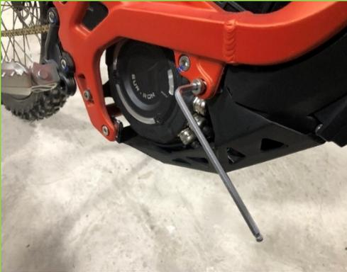
Step 2: Remove controller protection guard
