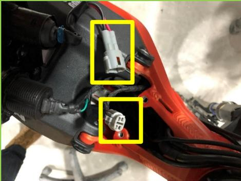
Step 3. use a short wire, make sure its conductive, and make sure you are safe
