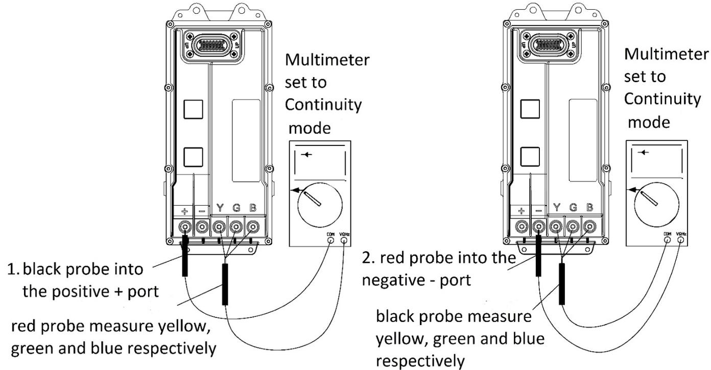
3. measure result should be between: around 0.2 and 0.6, can not be 0
