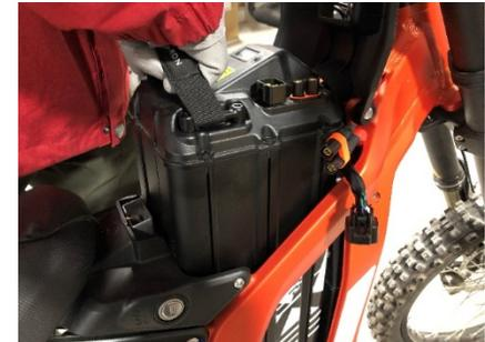
Step 2: Open the front battery plate
