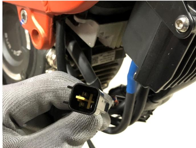
Test the bike after disconnect 12V converter, If the electric motor back to functional, then we can confirm that the 12V converter was malfunction.
