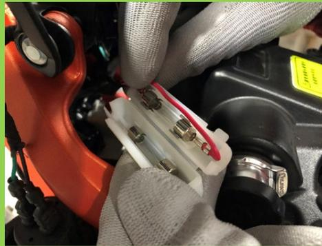
Step 3. check fuse, replace new fuse if blown.
