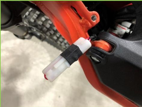
Step 2: open main fuse box, one is connected to main wiring loom, another is backup fuse
