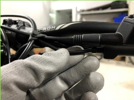
Step 2: remove the ignition key switch cap, find the sensor plug and disconnect the plug. Put the bike on the stand, lift the side stand, test the bike, if the motor back to work, then we can confirm the brake power protection malfunction, replace new part to repair.
