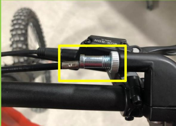
Throttle cable too tight, turn on switch will trigger protection
