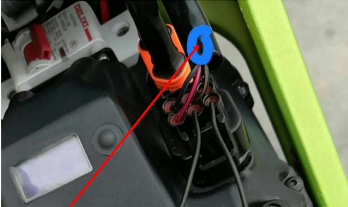
Inside of the bigger black wire protection rubber tube (which is marked in blue circle in the picture.), there's a wire was cut off. Please cut the bigger black wire rubber protection tube, connect the wire, then, you will have power and speed release.
