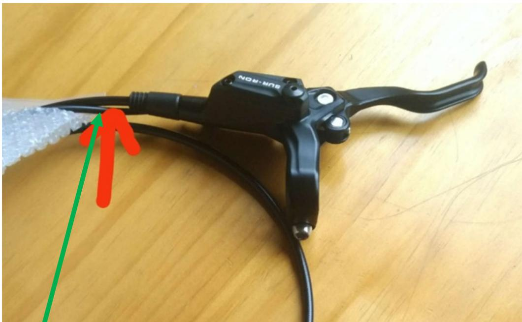
As above picture, there are two brake cable. The thick cable is for oil pump. The thin one is for brake power cut off protection (it means, when the riders use the brake, the power will be cut off, the bike will stop running). This protection is mainly for new riders, and consider about the safety.
